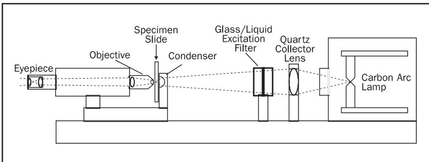
in gelatin, a chamber of liquid copper sulfate, and blue-violet colored filter glass. This first excitation filter produced a wide band of near-UV light with relatively little visible light, enabling the microscopist to observe the inherent primary fluorescence of specimens. Microscopists were aided by the fact that most substances will fluoresce readily when excited by UV light. In 1914 fluorochromes were first used with
