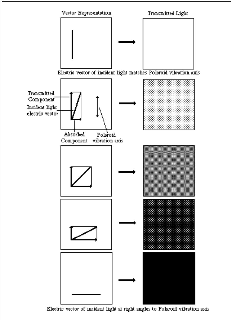
Figure 11.2 - Action of a Polarizer.
