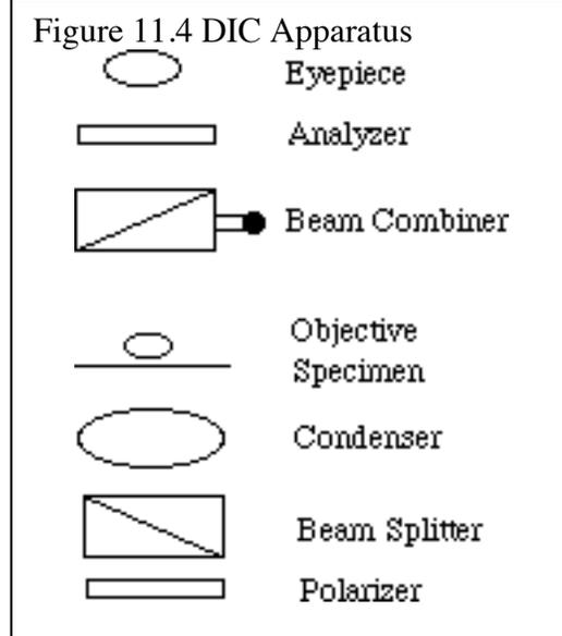
slightly sheared beams on the specimen plane. DIC requires that the microscope be aligned for Köhler illumination.
