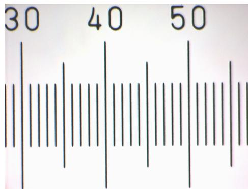
Figure 8.3 Image of a stage micrometer taken with a 20X / 0.75 objective lens. The line spacing is  $10 \mu\text{m}$ .
