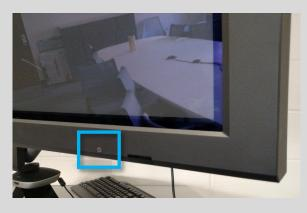
To turn on the television, press the **POWER** button located at the bottom side of the television. The television is meant to be used with the Video conference system to view content and far sites.
