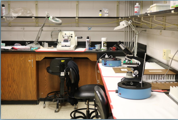
HRCF is equipped with two Leica RM2335 microtomes, microscopes and waterbaths, which are used to produce high quality paraffin tissue sections.
