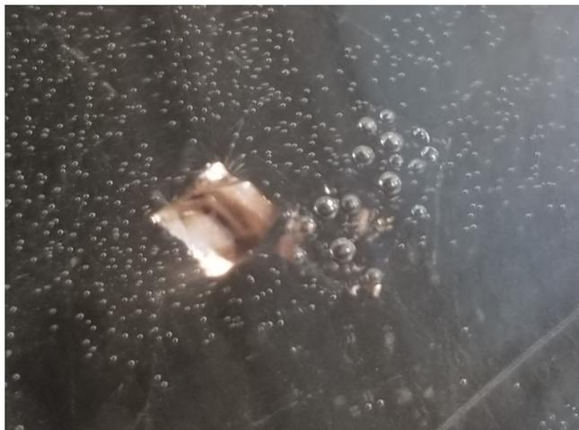
8. At this point you should have clear MMA/graphene films with the MMA layer facing up.
