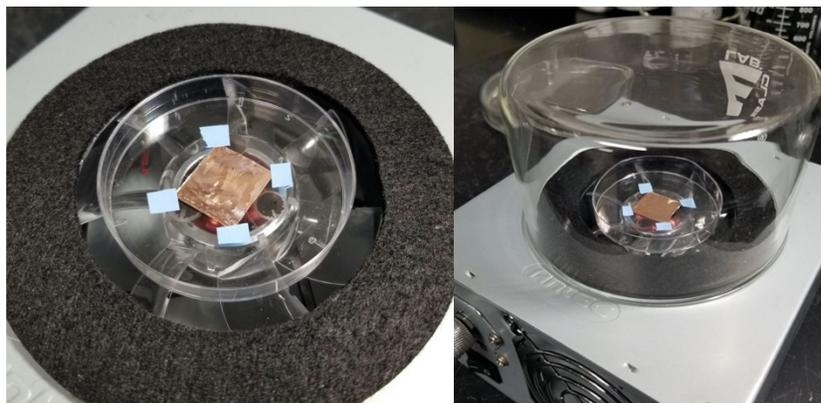
3. Place graphene/copper foil in spin coater, tape down corners. There is graphene on both sides of the copper foil, so it doesn't matter at this point which side is up.
