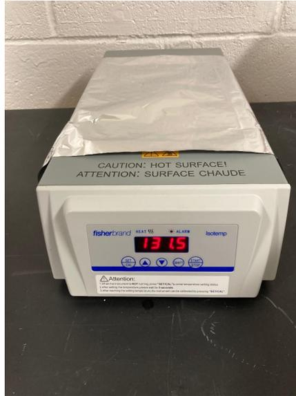
12. Place the grids warm acetone for 45 minutes, use small Pyrex dish, keep the TEM grids carbon side up.
