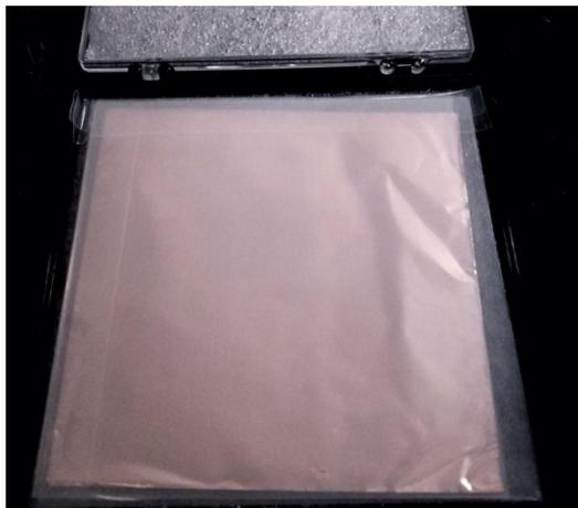
2. Cut out a section of graphene/copper film with enough area to cover the number of grids you intend to make. Use the small scissors to cut along the plastic film (use as a guide to make a straight line).
