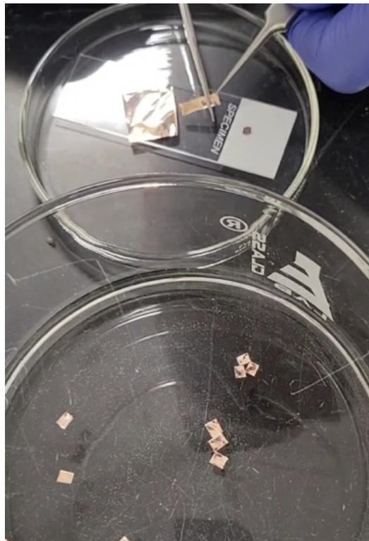
7. Float the newly cut pieces in 1 M ammonium persulfate (APS), exposed copper side down, to remove the copper substrate. This will take 1-2 hours. If, after 1 hour, some of the pieces still have a lot of copper, they were likely put on the surface of the solution upside down. Flip them over and let them sit for the remainder of the time or until no traces of copper are left on the films. The picture below shows a piece that was put in correctly (the large
