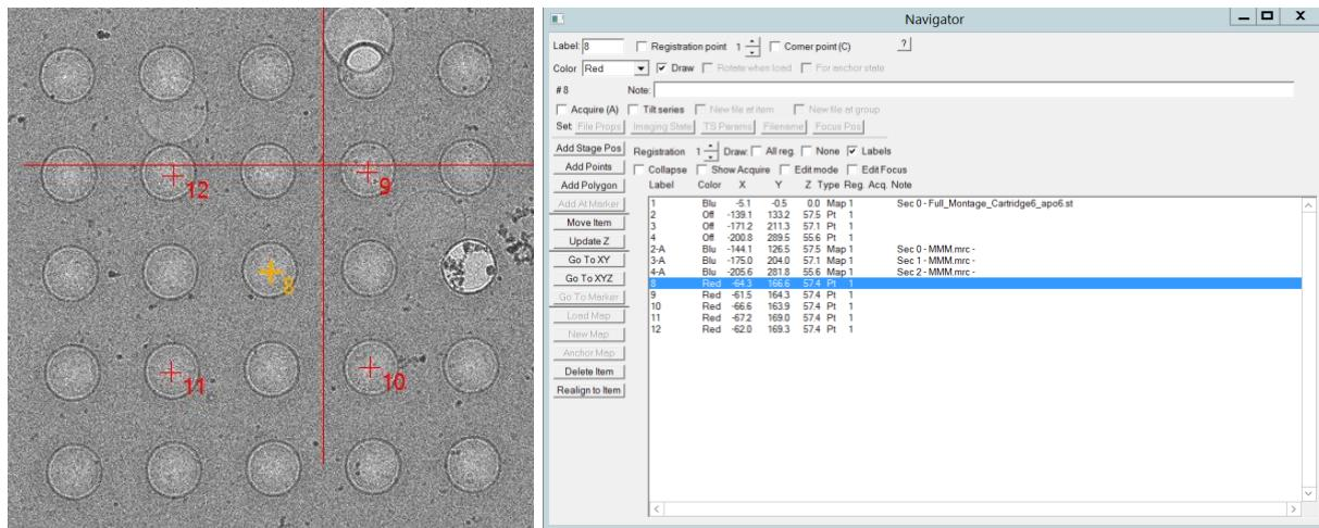
Take view of center point. If point is away from center hole (# 8 as shown), place marker in center of hole, navigator → shift to marker → “OK”
