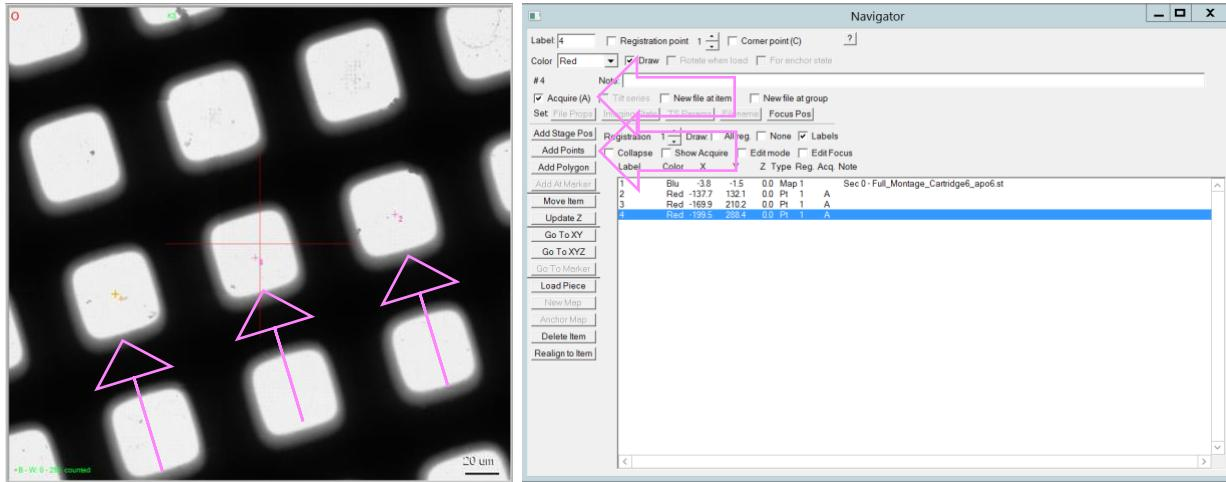
Find eucentric height (once at one grid square) using stage Wobbler on the microscope computer and “Update Z” for Acquire points (Purple arrow).
