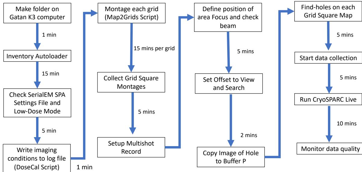
1. On the Gatan K3 computer make a new folder in the X: directory to save your data. **Make sure that the X: drive has enough free space if it is full delete old data.** Make sure the data has been fully transferred to the longleaf cluster or the NAS before deleting the data.
