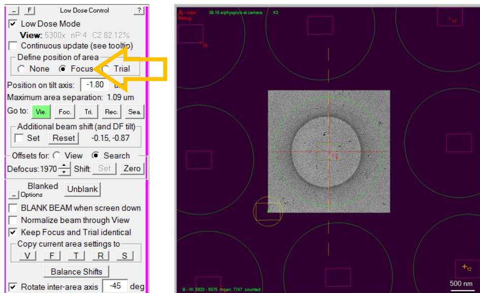
**At this point Focus beam is over the carbon and not illuminating the hole.**
