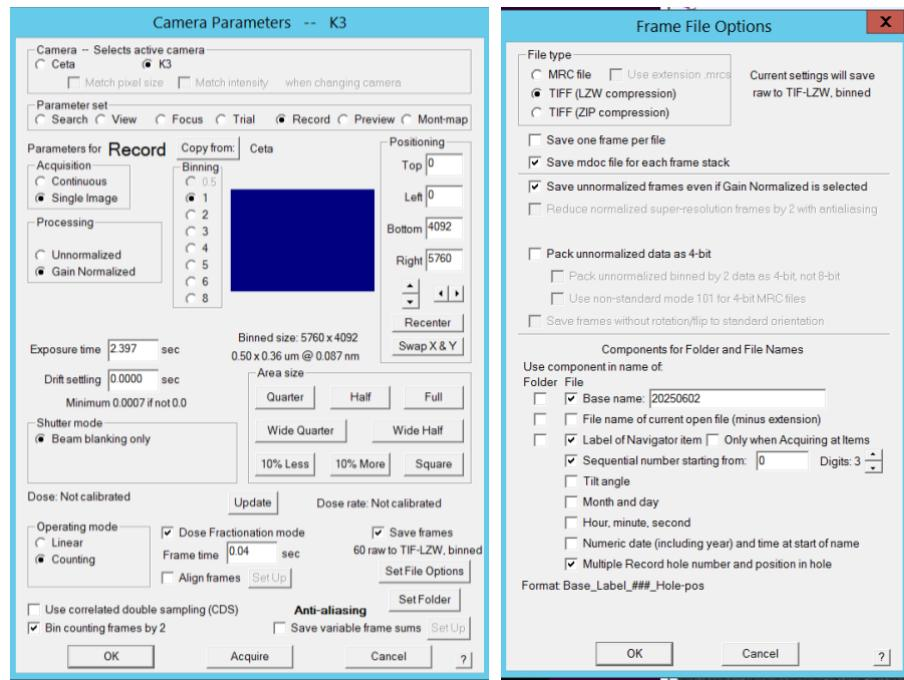
Navigator → acquire at items → final data → run script “DataCollection\_V6”, run script before action Multishot\_Filter\_Threshold → GO (couple hours)
