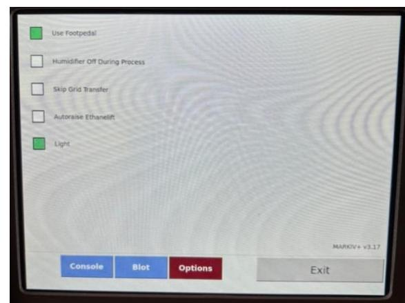
We recommend turning the humidifier off and set the temperature. It normally takes ~ 30 mins to cool the Vitrobot to 4 °C. Once the Vitrobot is cool, set the humidity to 95%. It normally take ~ 5 mins to reach high-humidity. **We recommend letting the Vitrobot filter paper sit in the chamber at high-humidity for ~ 1 hour before preparing cryo-grids.**
