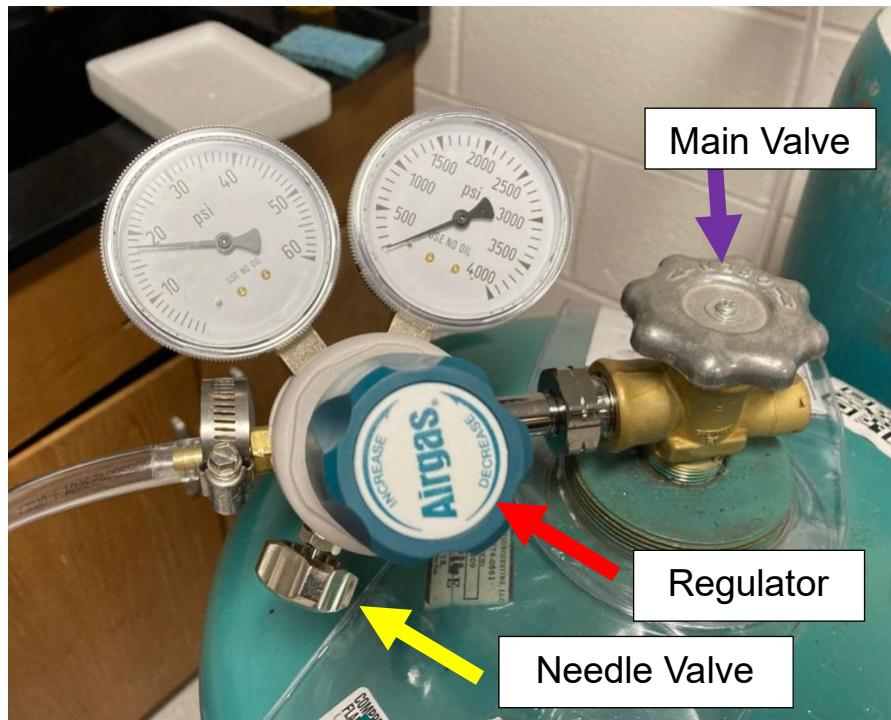
Before dispensing the ethane propane mixture, place the needle tube inside the ethane cup, orientate the tube at an angle touching the bottom of the ethane pot. Then open the needle valve to dispense the ethane propane gas. The gas should flow out slowly and will condense inside the ethane cup. Fill the pot the top, the level of ethane propane should be just below the spider. **When you are finished using the ethane propane, make sure to close the needle valve.**
