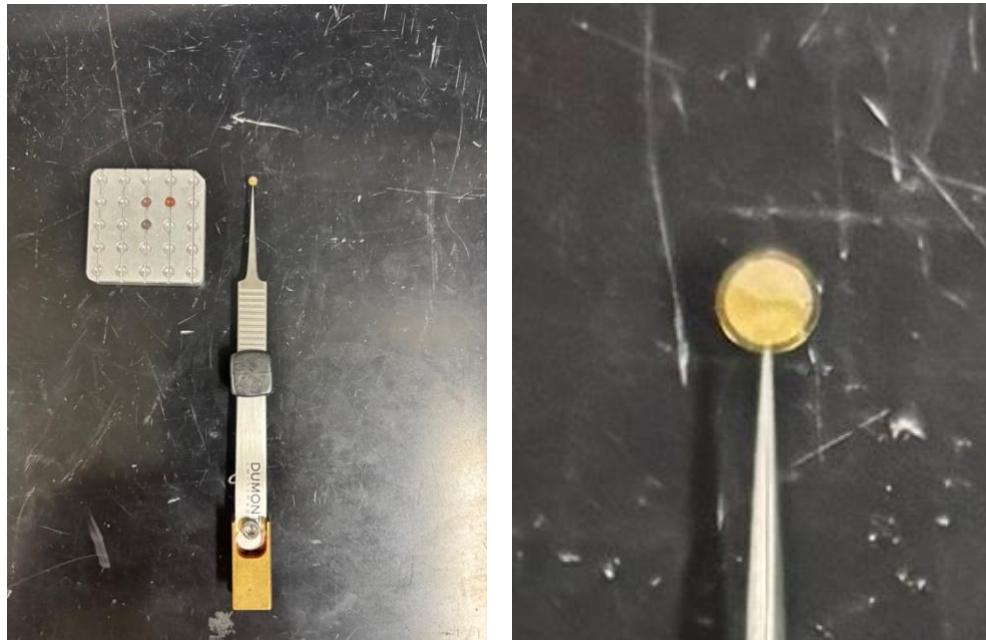
I am right-handed, I prefer to pick-up the TEM carbon side facing the Right Sample Port of the Vitrobot. Make sure the grid is not bent or damaged.
