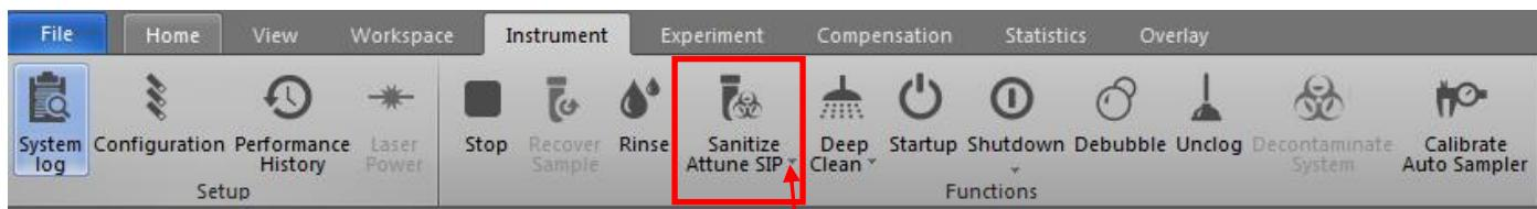
3. If the Autosampler was used, click on the small triangle and select **Auto sampler SIP**.
