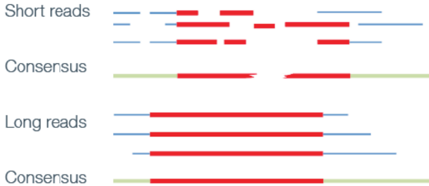
Figure 1: Long read lengths are more likely to incorporate the whole repetitive region (shown in red) allowing more accurate assembly with fewer gaps.
