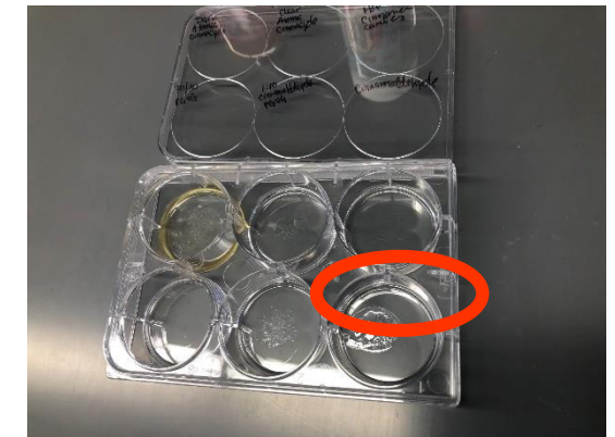
Red circle: corrosive effect of cinnamaldehyde electronic cigarette solution on plastic after 2 hours. Photo from Dr.
