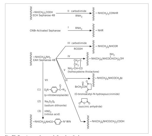
Fig. 72. Reactions used to couple ligands to Sepharose.
