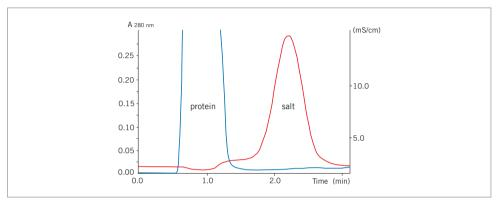
Fig. 76. Buffer exchange of mouse plasma (10 ml) on HiPrep 26/10 Desalting.
