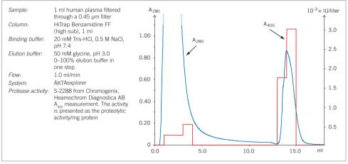
Fig. 31. Removal of trypin-like serine proteases from human plasma using HiTrap Benzamidine FF (high sub), 1 ml.
