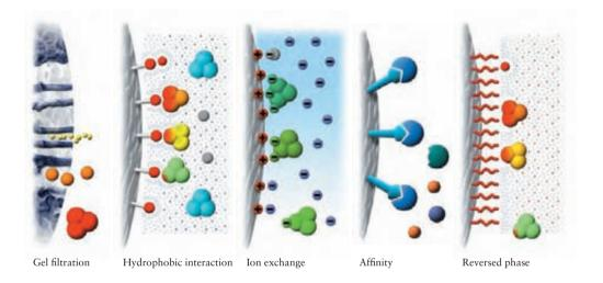
Fig. 1. Separation principles in chromatographic purification.
