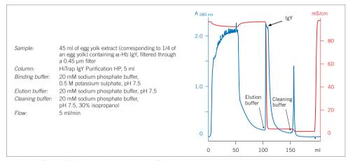
Fig. 20. Purification of avian IgY on HiTrap IgY Purification HP.
