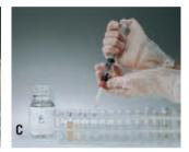
Fig. 16. Using HiTrap Protein G HP with a syringe. A: Dilute buffers and prepare sample. Remove the column's top cap and twist off the end. B: Equilibrate the column, load the sample and begin collecting fractions. C: Wash and elute, continuing to collect fractions.
