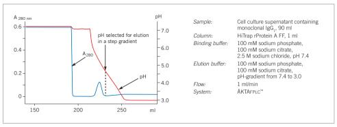
Fig. 8. Scouting for optimal elution pH of a monoclonal IgG, from HiTrap rProtein A FF, using a pH gradient.
