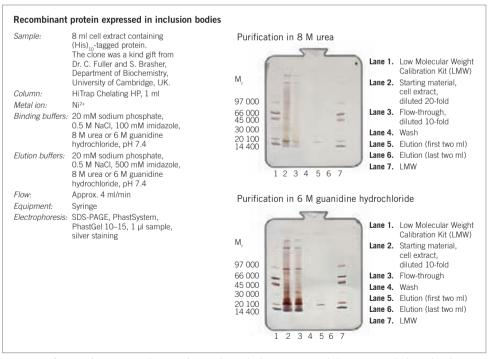
Fig. 26. Purification of (His)<sub>10</sub>-tagged protein from inclusion bodies on HiTrap Chelating HP, 1 ml, charged with Ni<sup>2+</sup>.
