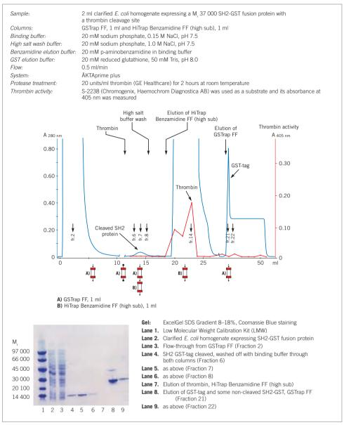
Fig. 32. On-column cleavage of a GST fusion protein and removal of thrombin after on-column cleavage, using GSTrap FF and HiTrap Benzamidine FF (high sub).
