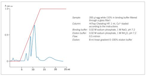
Fig. 49. Purification of egg white proteins on HiTrap Chelating HP 1 ml, using the metal ion Cu<sup>2+</sup>.
