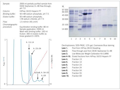
Fig. 37. scCro8 purification on HiPrep 16/10 Heparin FF.
