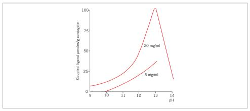
Fig. 69. pH dependence of coupling N-acetyl-D-galactosamine to Epoxy-activated Sepharose 6B. Carbonate/bicarbonate buffers were used in the range pH 9–11, sodium hydroxide solution in the range pH 12–14. Ligand concentrations: 5 mg/ml and 20 mg/ml.
