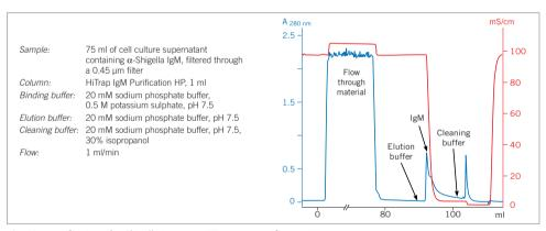
Fig. 19a. Purification of  $\alpha$ -Shigella IgM on HiTrap IgM Purification HP.
