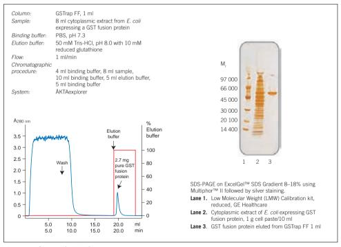
Fig. 22. Purification of a GST fusion protein.
