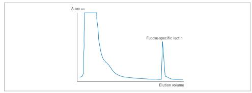
Fig. 68. Chromatography of a crude extract of *Ulex europaeus* on fucose coupled to Epoxy-activated Sepharose 6B, column volume 11 ml. Extract was applied in 0.9% NaCl. Fucose-specific lectin was eluted with 5 ml fucose (50 mg/ml).
