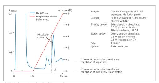
Fig. 7. Gradient elution of a  $(His)_6$  fusion protein.
