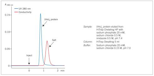
Fig. 77. Desalting of a (His), fusion protein on ÄKTAprime plus.
