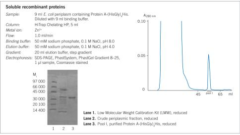
Fig. 25. Purification of recombinant proteins on HiTrap Chelating HP, 5 ml, charged with Zn<sup>2+</sup>.
