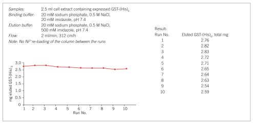
Fig. 50. 10 repetitive purifications of GST-(His), without reloading the column with Ni<sup>2+</sup> between the runs.
