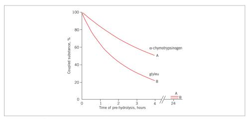
Fig. 63. Variation of coupling activity with time of pre-hydrolysis at pH 8.3. CNBr-activated Sepharose 4B was washed at pH 3 and transferred to 0.1 M NaHCO<sub>3</sub>, pH 8.3 for pre-hydrolysis. Samples were removed after different times and tested for coupling activity towards α-chymotrypsinogen (A) and glycyl-leucine (B).
