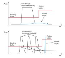
Allow time for the sample to bind and/or apply sample in aliquots, stopping the flow for a few minutes between each sample application (see second figure beneath).
