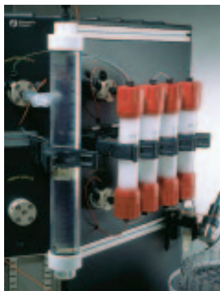
Fig. 51. Four HiPrep 26/10 Desalting columns connected in series.
