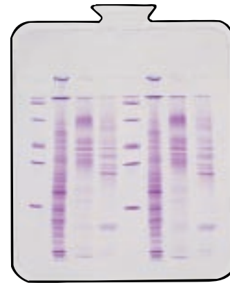
Fig. 3. Example of native PAGE with PhastGel gradients 8–25. The gel was Coomassie stained as described in development technique file number 200. Starting from the left, the four repeating samples are: HMW Calibration Kit, proteins, E. coli , salmon extract, and coalfish extract.
