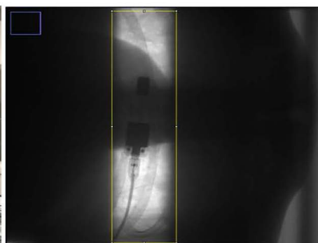
Figure 1 b: Entrance dose measurement within the collimated field with the RF probe
